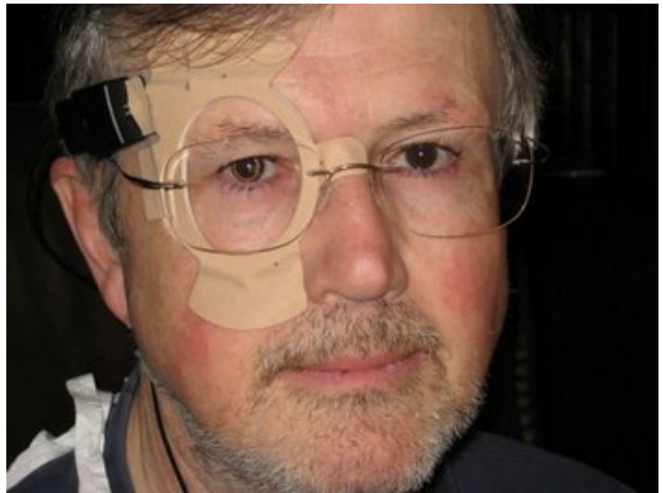
Jacqueline Grau David Grau of San Diego wears a high-tech Triggerfish contact lens in his right eye. The silicon wafer is ringed with circuitry that measures pressure changes in the eye and transmits the data to a receiver worn next to the ear.
